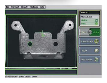
The new MotoSight2D Vision combines leading vision technology with leading robotic technology. The MotoSight2D product range is based on compact 2D cameras in 3 different performance classes. In addition to simple data exchange, programming of the camera from the teach pendant of the robot is also possible.
